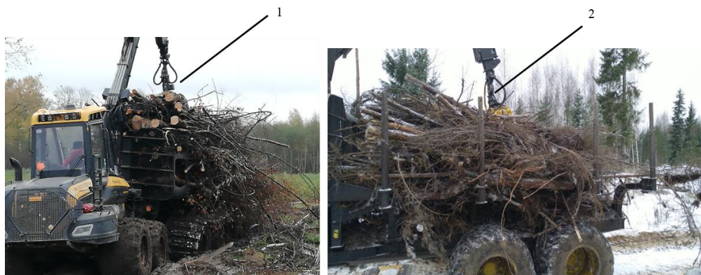
Fig. 1. Weighing systems used in the study: 1 – Intermercato scale; 2 – JohnDeere scale
